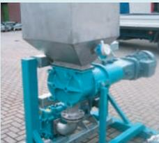
**Slaughterhouse Waste** needs to be macerated and transferred. A customized package includes a receiving hopper, a side mounted Multicrusher with increased suction opening and a Rotary Lobe Pump. The system is extremely compact, but still easy to maintain with Börger MIP-Design.
